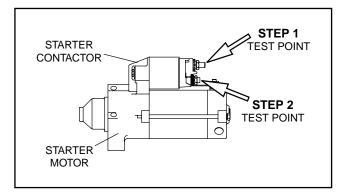
Figure 9. The Starter Contactor (V-twin Units)
